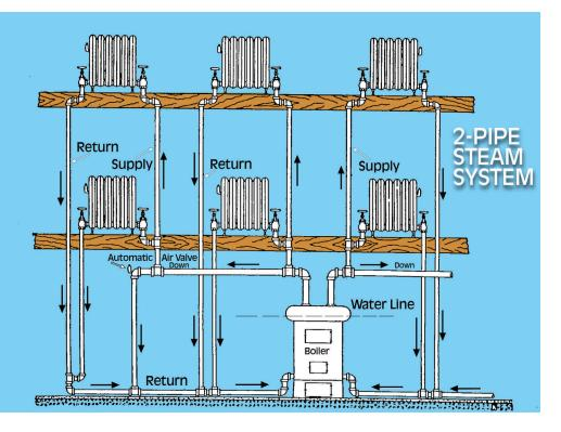
allowed to help the returning condensate get back into the bottle. But when the thermostat says it's had enough, it tells the zone valve to close and there is no longer any leftover steam pressure to help the returning condensate. Without the pressure, the returning condensate is forced to back up the return piping and enters the steam main, trying to develop enough pressure (through stacking).
