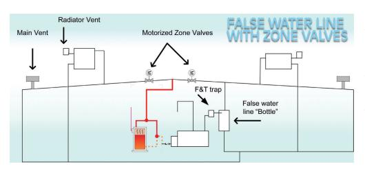
portion of the wet returns, which would create incredible banging and clanging noises. The key to a successful false water line installation is to mount the bottle or large Float & Thermostatic trap (F&T) at the water line height of the original boiler. That way, you are assured that all of the original piping that was wet remains wet and everything above the old boiler's water line stays dry. (See Figure 2)
